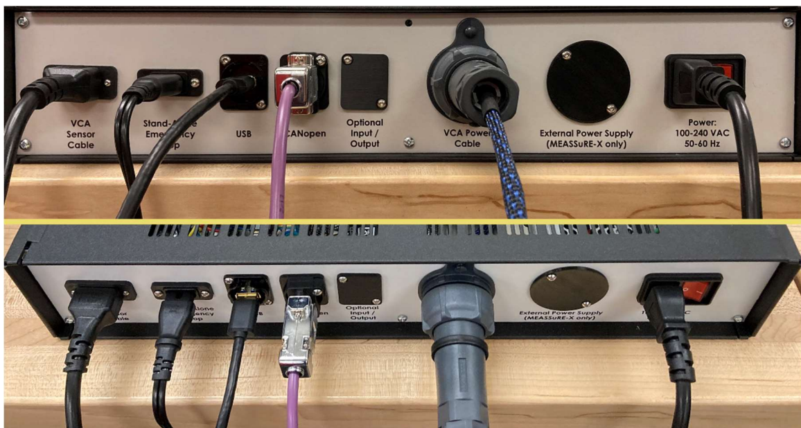
Fig. 5: Front and top view of the electronics enclosure's rear panel with cables connected.
