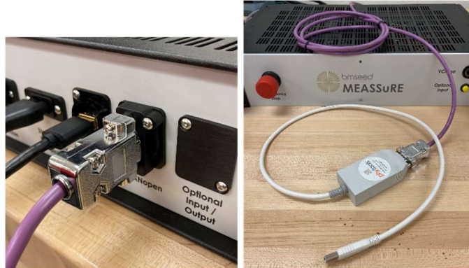
Fig. 4: PCAN extension cable (purple) connected to the "CANopen" connector on the enclosure and the PCAN-USB adapter (white) to be connected to the computer.
