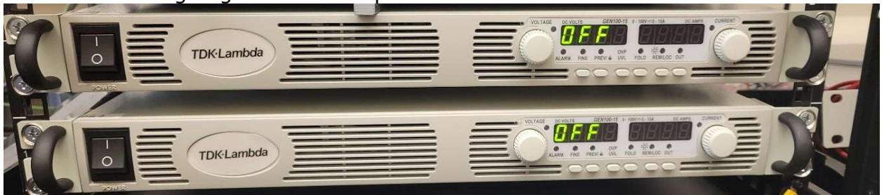
Fig. 7: Power supplies after turning on pressing the power switch on the left.
