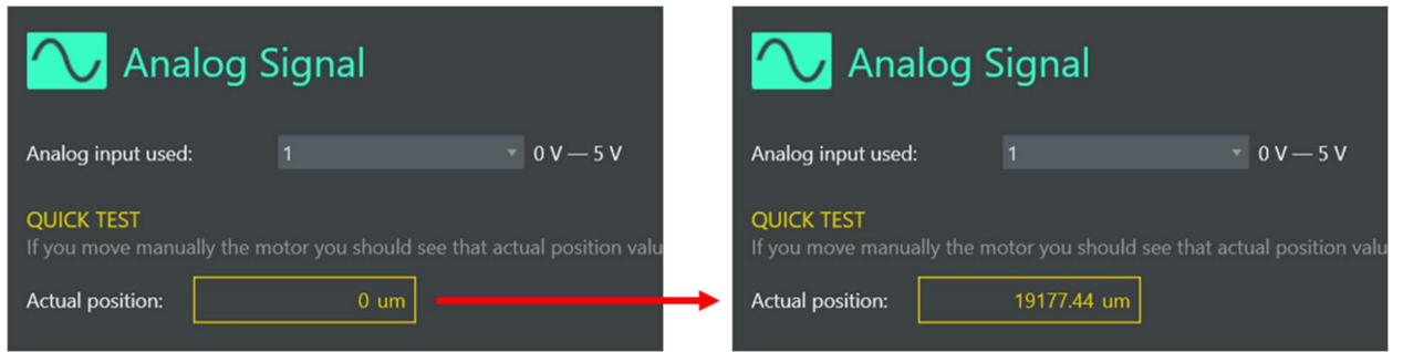
Fig. 26: Testing the actual position (i.e., analog signal) of the VCA.
